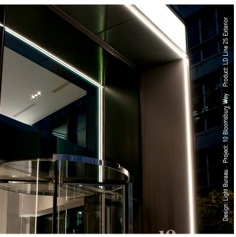
The new LD Line 25 is an exterior rated LED homogenous line of light. It is custom made to suit the dimensions on site. Cut increments of 50mm allow lengths to fit into most details, with minimal dark spots. Please note that LD Line 25 Exterior is not suitable for external applications within the floor / ground. LD Line 25 can be mounted internally into the floor / ground, but only in areas of low footfall.
